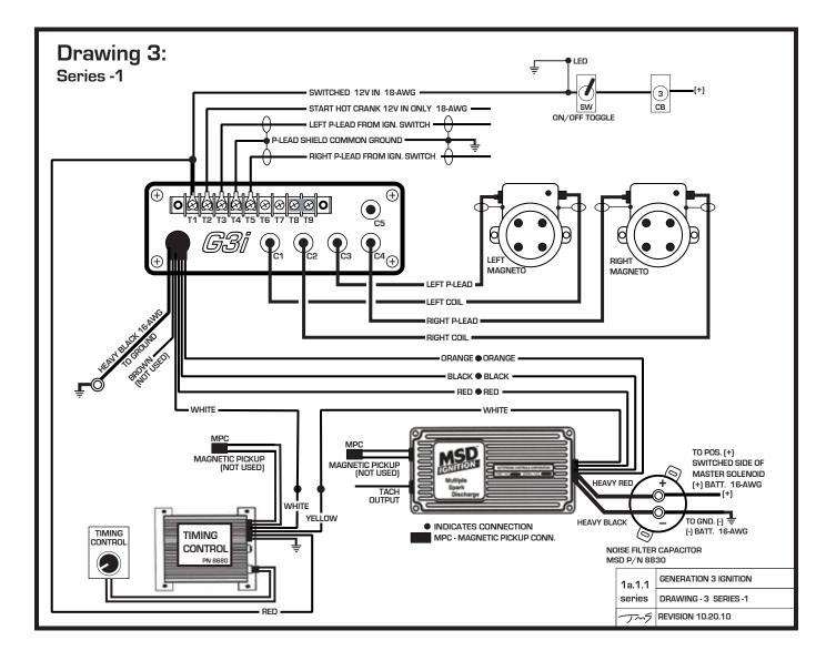
Left Magneto Normal Contacts are Trigger Source Left Magneto Lag – Retard Impulse Coupler MSD 8680 Adjustable Timing Control \*\*\* BRIDGE TERMINALS (T8 - T9) \*\*\* G3i White lead is routed to White lead on MSD 8680 Adjustable Timing Control.
