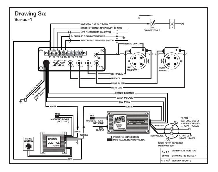
Left Magneto Normal Contacts are Trigger Source Left Magneto Retard Contacts / Active in Start MSD 8680 Adjustable Timing Control \*\*\* BRIDGE TERMINALS (T6 - T7) (T8 - T9) \*\*\* Retard Contact P-Lead to BNC (C5) G3i White lead is routed to White lead on MSD 8680 Adjustable Timing Control.
