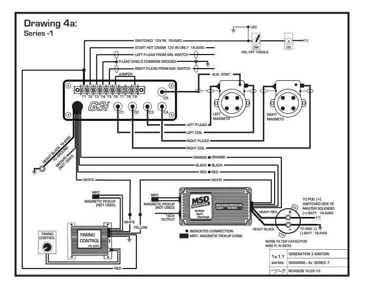
Left Magneto Auxiliary Contacts are Trigger Source Left Magneto Lag – Retard Impulse Coupler Starting on Normal Contacts MSD 8680 Adjustable Timing Control \*\*\* BRIDGE TERMINALS (T6 - T9) (T7 - T8) \*\*\* Auxiliary Contact P-Lead to BNC (C5) G3i White lead is routed to White lead on MSD 8680 Adjustable Timing Control.
